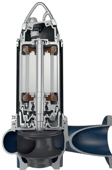
FIGURE 4.29 Submersible pump. (Courtesy of Grundfos.)
